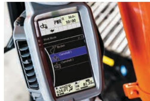
Switch between workmodes via the monitor.
