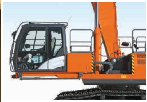
The sliding cab enhances visibility and safety.
