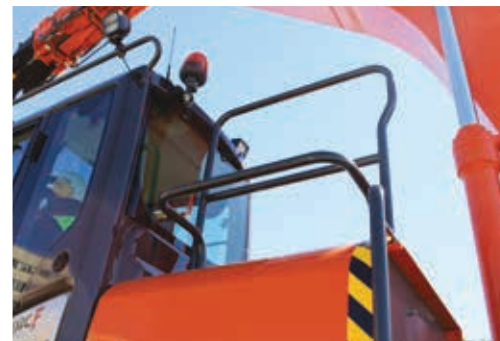
A long step and handrails enable safe access to the cab.
