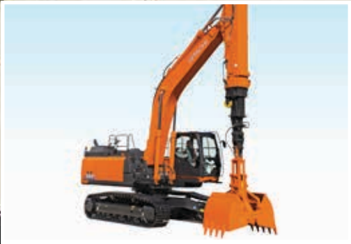
The telescopic arm extends and retracts smoothly with a full load.
