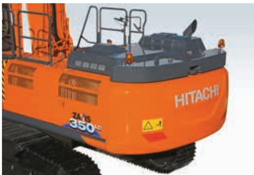
The detachable counterweight enhances the machine's versatility.
