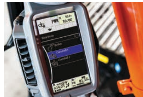
Switch between workmodes via the monitor.
