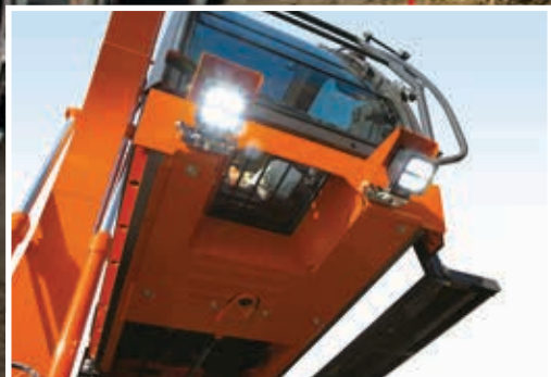
Optional LED lights highlight the working area for operators.
