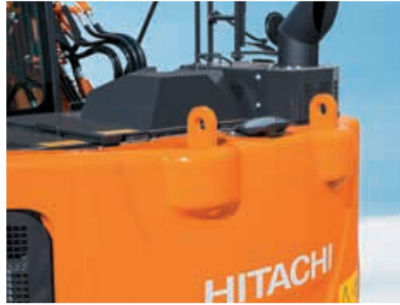
Brackets on the upper structure for safe lifting.
