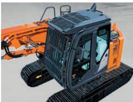
Front top guard complies with demolition specifications.
