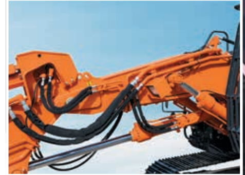
Enhanced hydraulic circuit for use with larger attachments.
