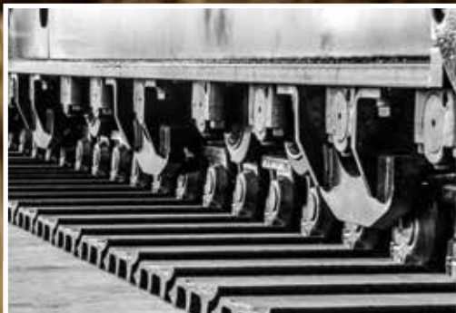
More track guards enhance the durability of the track link.
